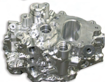
Comparing the design model to the VERICUT “as machined” model helps Tell Tool locate gouges.
