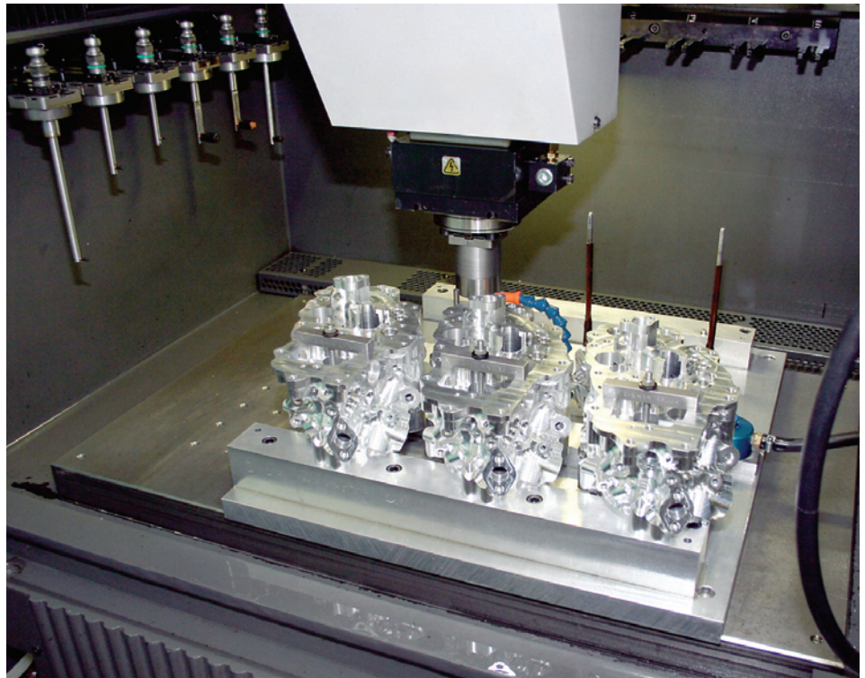
To eliminate chatter and improve surface finishes, the company uses VERICUT's OptiPath module to determine the appropriate feed rates.
