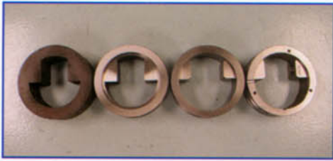
Pictured from left to right: Part after water jet and heat treat, part after lathe turning, part after wire EDM, and finished part.
