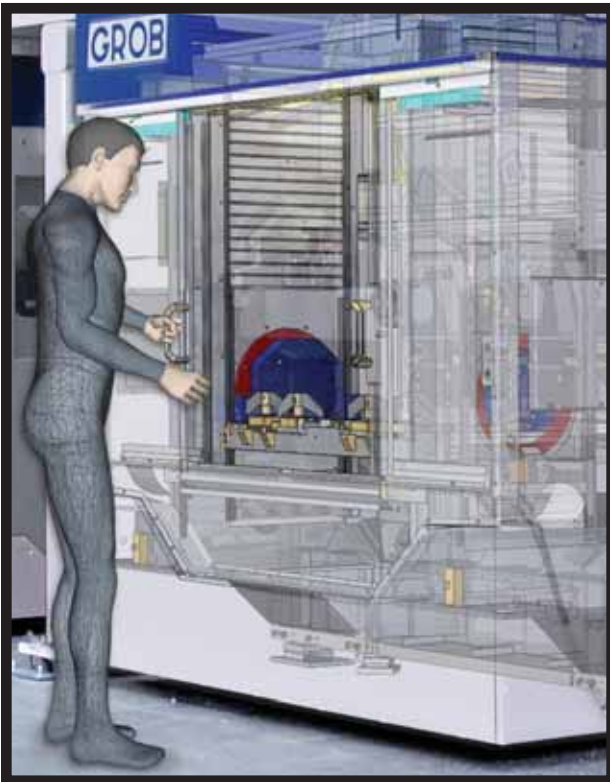
New Jack human modeling in Siemens PLM Software's Tecnomatix 9 adds realism to simulations.
